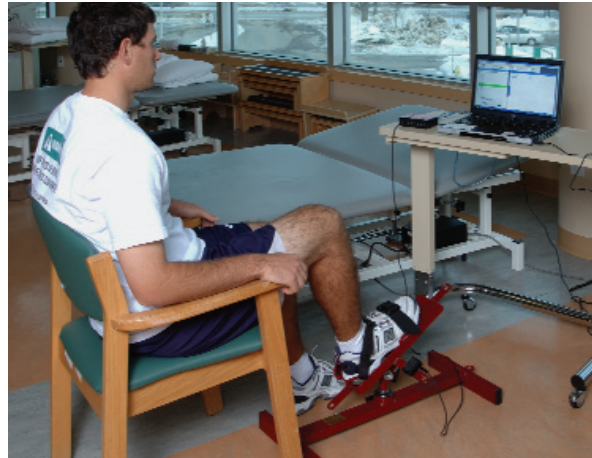
Figure 1: A patient can play a computer game to practice ankle flexion and extension using the NeuroGym ® Trainer biofeedback with position sensors.
